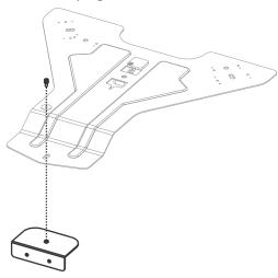
8. For 630-GS and 635-GS only, install the rubber spacer provided in the installation kit on top of the default rubber spacer on the lens support bracket.
