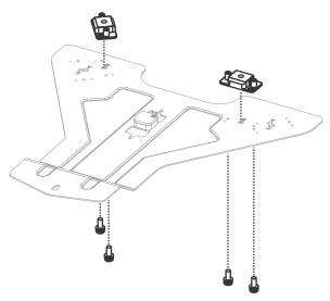
7. To secure the angle bracket to the lens support bracket, install one M3x8 hex screw and one M3 washer.
