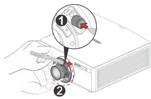
2. Remove the lens through the front of the projector.
