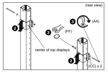
Use 5/16-18 x 4 1/2" button head cap screw (AA), two 5/16" washers (CC) and 5/16-18" lock nut (FF) to secure each clamp bracket (P) to column. (See Figure 5)
