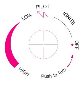
5. After depressing the control knob for 30 seconds, turn control knob to LOW.
