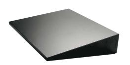
This Wall Mount Shelf is an ideal solution for wall mounting any nonrackmount equipment in a wide variety of applications from small IT installs to colocation datacenters. This shelf will support up to 120lbs of evenly distributed weight with its steel construction. Six keyhole openings on the rear of the shelf for mounting are spaced 16in on center for standard wall studs.
