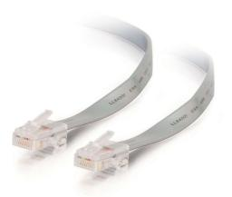
Constructed from heavy duty 26 AWG silver satin wire, this crossed modular cable is ideal for voice, telephone and modem communication applications. has gold-plated connectors for clearer communication. This cable is also known as a "rollover" cable which is commonly used when configuring routers.
