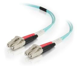
This OM4 Duplex Multimode Fiber Optic Cable is ideal for connecting 40GBase BiDi 10GBaseSR, SFP+ and QSFP+ transceivers for 40 and 10 Gigabit network connections. This cable provides backward compatibility with existing 50/125 equipment and the performance headroom required to support LED and VCSEL laser light sources, and 40 or 10 gigabit Ethernet applications in a datacenter or wiring closet..
