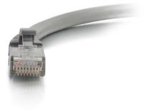
This Snagless Unshielded Cat6a patch cable is ideal for use with 10GBase-T ports and equipment, such as network adapters, hubs, switches, routers, DSL/cable modems and patch panels, and enables 10 Gigabit data transmission over a 4 pair copper cable allowing connections up to 100 meters. Current Cat6 cabling systems may only support 10 Gigabit Ethernet over limited distances. Each patch cable is fully tested to meet ANSI/TIA 568 C.2 Cat6a channel requirements.
