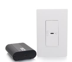
C2G Superbooster USB Extenders deliver reliable USB signal transmission for USB devices, allowing devices such as cameras, interactive whiteboards and printers to be placed at greater distances from the host computer.
