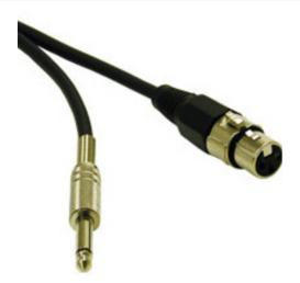
Use this XLR to 1/4in cable to connect microphones and balanced sources to unbalanced inputs. This pro-audio cable is made from 22 AWG twisted pair audio cable under an aluminum foil shield and 60% copper braid for maximum shielding from noise. The highly flexible 7mm PVC jacket reduces the risk of the cable kinking and damaging the conductors.
