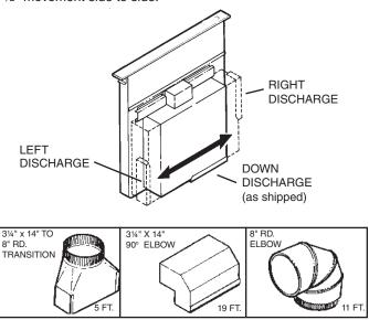
The system will operate most efficiently when the ductwork does not exceed 40 feet of equivalent duct. The chart above, shows equivalent feet of elbows and transitions. The number of feet of straight 3½" x 14" or 8" duct plus the equivalent feet of elbows or transitions to be used should equal 40 feet or less.
