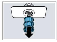
4. Press the locking catches ① together and take the coarse filter upward and out ②.
