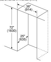
Leave 1/2" (12.7) gap at the top and 1" (25.4) behind the refrigerator for proper ventilation.
