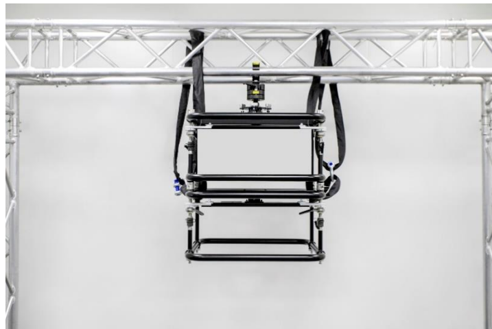
Figure 21 Securing two frames with two sets of rigging slings
