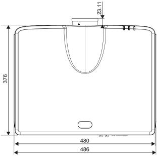
Image A-2 Dimensions given in mm
