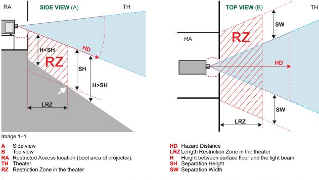
Based on national requirements, no person is allowed to enter the projected beam within the zone between the projection lens and the related hazard distance (HD). This shall be physically impossible by creating sufficient separation height or by placing barriers. The minimum separation height takes into account the surface upon which persons other than operator, performers or employees are permitted to stand.
