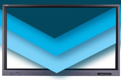
The cutting-edge lightweight LED technology of the Avocor E series 65" interactive display combines first-to-market 2mm optically bonded glass with a 4K IR interactive display. The E series delivers ultra-fast 20-points of touch using Avocor Intelligent Touch, the functionality to insert an OPS unit as well as the Connect and Control bar at the bottom of the screen.
