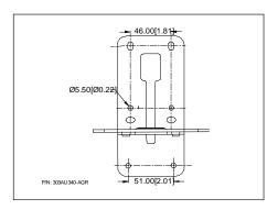
2. Use the screw to secure the A L-mount bracket on the wall.
