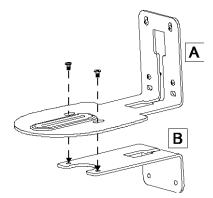
4. After assembling the L-mount bracket, secure the lower part of L-mount bracket on the wall.
