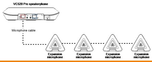
**[Note]** The VC520 Pro can support up to four expansion microphones, however, the daisy-chain expansion cable cannot exceed over 40m in total.
