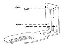
3. Then, assemble the  $\boxed{\mathsf{A}}$  +  $\boxed{\mathsf{B}}$  L-mount bracket with screws (included in package).
