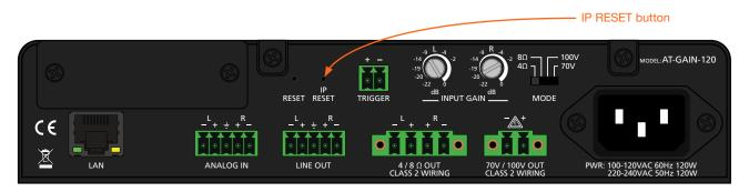
3. Release the **IP RESET** button once the **PWR** LED indicator on the front panel begins to flash. The number of flashes will indicate the currently selected IP mode.
