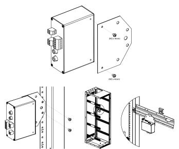
TSD-RMK Optional 19" Width Rack Mount Kit - For 19" rack mounting, Atlas Sound offers an optional rack mount kit, the TSD-RMK. This rack mount kit can support up to four TSD units. The kit includes three blank panels designed to fill any unused slots. Use the included hardware to mount the TSD into the rack mount kit using the top mount screw holes on the TSD.
