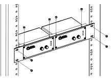
5. TSD-RRMK Optional Rear Rack Mounting Kit - For complete flexibility in mounting a TSD or TSD external power supplies the optional TSD-RRMK is available. The TSD-RRMK can support mounting of either two larger TSDs with external power supplies or up to 4 TSD models. Note: Only use the included M3 x 4mm screws as other screws may be too long and will cause internal damage to the TSD.
