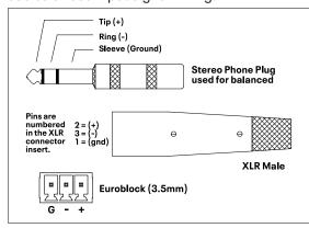
Each channel's Euroblock, 1/4" phone jack, and XLR inputs are wired in parallel, with XLR pin 2 (+) and pin 3 (-). When using an unbalanced input, wire the signal to the input (+) Euroblock pin, phone jack tip, or XLR pin 2, and also be sure to wire the input (-) pin, phone jack ring, or XLR pin 3 to ground. Do not leave the (-) input unconnected. Avoid running low
