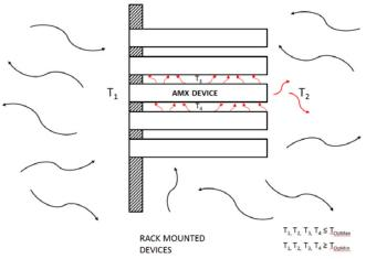
FIG. 6 HEAT CONVECTION IN RACK-MOUNTED DEVICES
