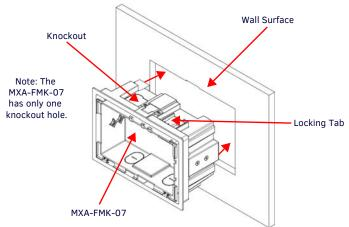
FIG. 3 INSERTING THE MXA-FMK-07 INTO THE WALL SURFACE (LANDSCAPE)
