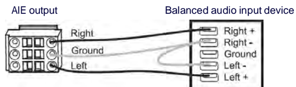
FIG. 111 Wiring from AIE to balanced audio input device if buzzing occurs
