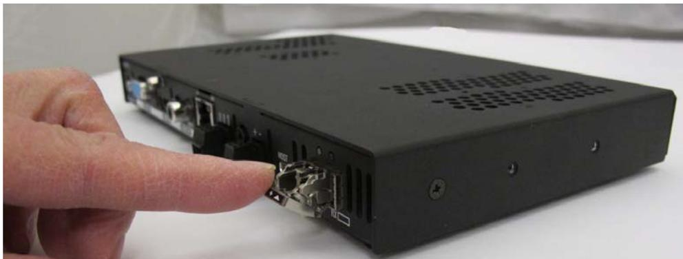
**FIG. 64** Flip transceiver latch out and down (DXLink Fiber Transmitter shown)
