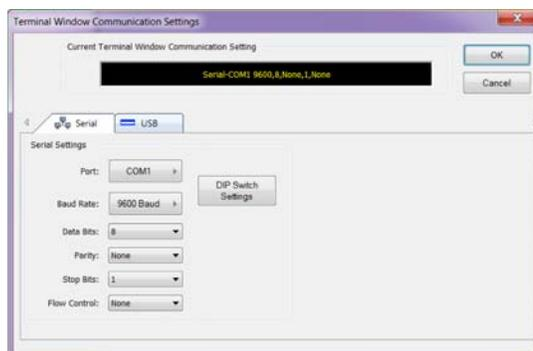
4. Set the COM port and the Serial Settings (Enova DGX default settings: 9600 Baud / 8 / None / 1 / None).
