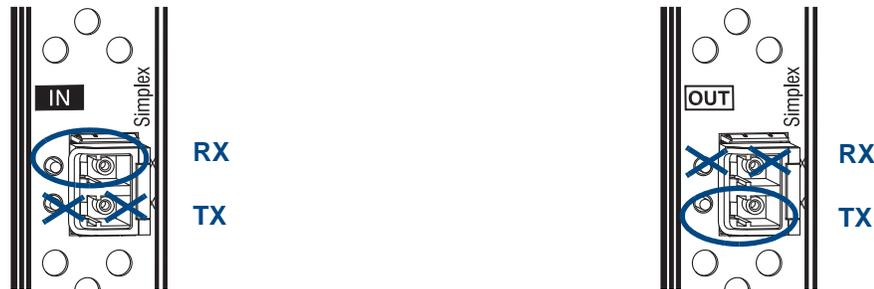
FIG. 59 Fiber optic transceiver LEDs on DXLink Fiber, Simplex Board (Enova DGX 32)
