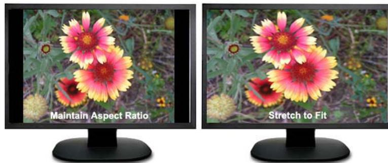
**FIG. 107** Example of displays set to Maintain Aspect Ratio and Stretch to Fit
