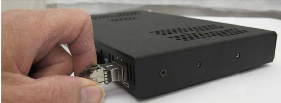
**FIG. 65** Pull transceiver free from transceiver socket
