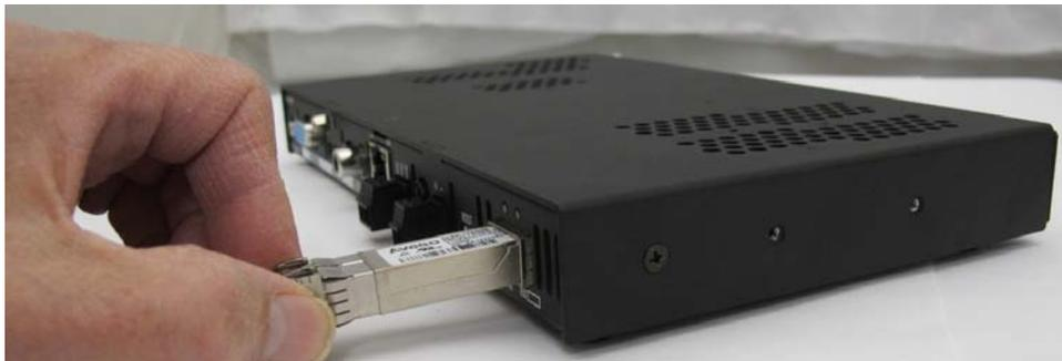
**FIG. 66** Insert transceiver into transceiver socket
