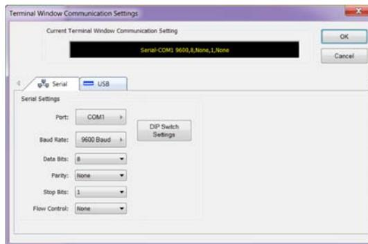
5. Set the COM port and the Serial Settings (Enova DGX default settings: 9600 Baud / 8 / None / 1 / None).
