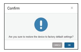
A successful reset will restore all the device settings to their factory defaults and the device will reboot automatically. Allow at least 2 minutes for the reboot to complete.
