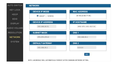
Allow 2-3 minutes for the device's LAN module to reboot and reconnect after the network setting is changed.
