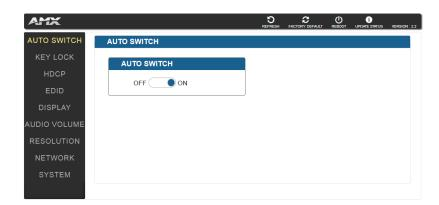
The Web UI page consists of several sections for basic and advanced settings: Auto Switch, Key Lock, HDCP Support, EDID Support, Auto Display Control, Relay Controller, Audio Output Volume, Output Resolution Setting, Network, Refresh, Factory Default, Reboot, Update Status.
