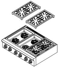
Grates are packed in a separate box. Inspect grates for rubber feet. Each grate must have four feet. Place grates on top of cook top.
