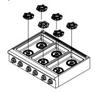
The open burner heads are packed in a separate box. Unpack and place the burner heads on the burner base. Align holes in the top burner with pins on the base of burner for proper capacity & operation. For locations of burner heads, see the diagram below.
