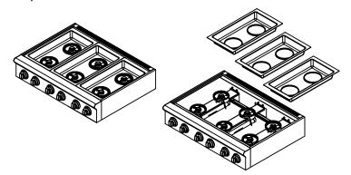
Remove the burner pans, then cut and discard the shipping ties on the burner base. Confirm that burner base is flat on the burner support and that the air shutter is positioned over the gas orifice. Replace the burner pans.
