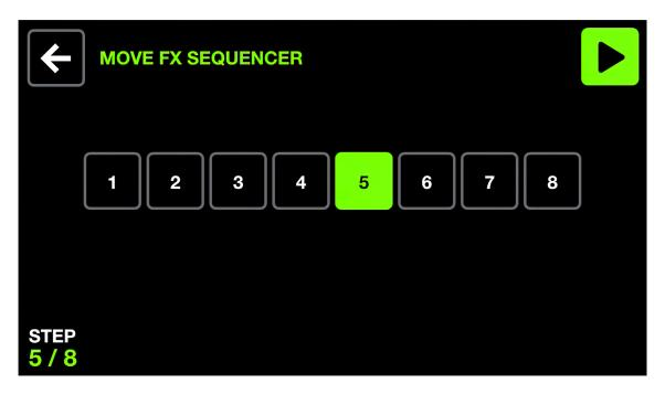
The Move Fx sequencer allows for eight different positions to be chosen. Each position will be played sequentially according to the FX speed.
