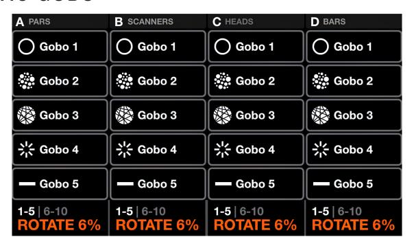
The static gobo screen contains a palette of 10 gobos per group. Selecting a gobo will recall the gobo on all fixtures in the group. If a gobo is not selected, the open gobo will be triggered.
