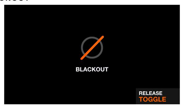
The Blackout flash effect shuts off all beams by setting dimmers to 0%, shutters closed, and color mixing channels to 0%. The effect is released according to the set release mode.
