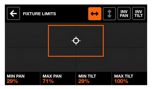
The fixture limits screen allows for minimum and maximum pan and tilt values to be set on the selected fixtures. When set correctly, fixture beams will move together in the desired area.
