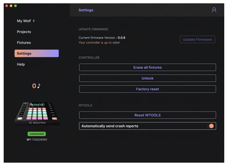
The Settings screen shows the current firmware version. Clicking Update Firmware will update to the latest firmware version which is downloaded automatically from WTOOLS when connected to the internet.
