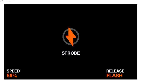
The Strobe flash effect tells all lights to strobe by triggering the fixtures strobe feature. If the fixture doesn't have a built in strobe feature, a virtual strobe will be created by flashing the RGB or dimmer channels. The effect is released according to the set release mode.
