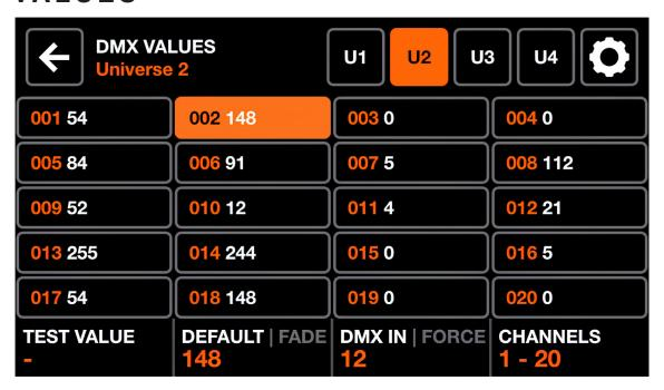
The DMX Values screen displays the current value of each DMX channel. It allows for the value to be changed for testing purposes, and for channel settings to be adjusted.
