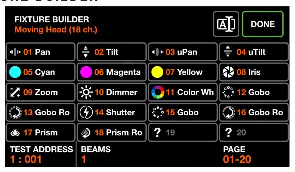
The fixture builder is used to create fixture profiles. A fixture profile is a list of channels and features associated with a particular fixture.
