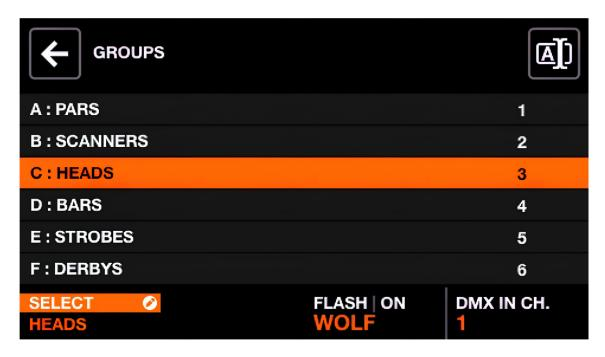
Each fixture is linked with a group. Effects, sub-dimmers, static colors and positions are applied to each group. Wolfmix supports up to 8 groups. 4 can be displayed at a time with groups A-D and E-H toggles by shift + hitting the BPM TAP button. Each group can be assigned a name and a DMX input channel on the Groups screen.
