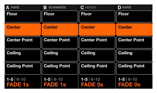
The static position screen contains a palette of five positions per group. Selecting a position will override any playing move effects on the group and set all fixtures in the group to the selected position.
