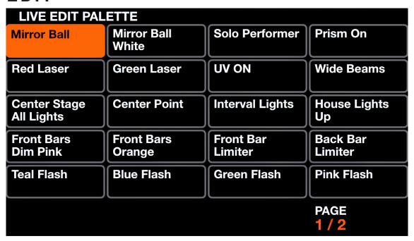
The Live Edit screen contains a palette of twenty buttons which can be used to recall a value on any channel. These values override all effects and other static values. Live Edits are layered in order, therefore if two live edits have values on the same channel, the buttons towards the bottom will take priority. Live Edits can also be released automatically by Row or Column and this can be set from the Settings screen.
