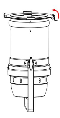
3. Return the retaining clip to the original position.
