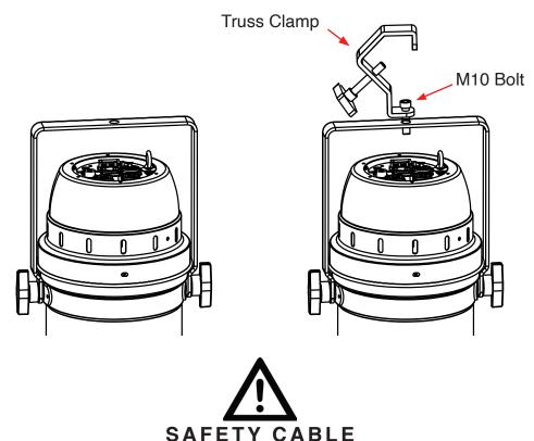
ALWAYS ATTACH A SAFETY WHENEVER INSTALLING THIS FIXTURE IN A SUSPENDED ENVIRONMENT TO ENSURE THE FIXTURE WILL NOT FALL IF THE CLAMP FAILS. CLAMP INSTALLATION
