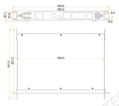
Tolerance: ±0.3 Unit: mm
