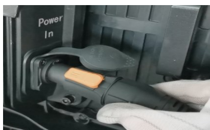
Power cable connection
