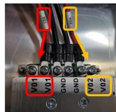
**When replacing the power supply, disconnect the main power supply to avoid electric shock;**
