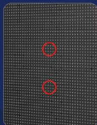
Insert tool into the maintenance hole
