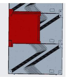
(2) Hang the middle row of boxes first, with the hook connection piece on the back of the box hooked into the groove of the back frame cross member profile. Move the box position so that it is centred and aligned with the marked line on the crossbeam;
