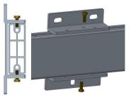
Once the corner yards are installed, fit the back hangers, using 2 M6\*16 in each position Screwed in place (screwed into a groove in the crossbar, clamped top and bottom)
