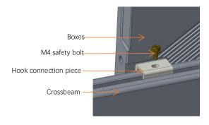
Note: The internal structure is based on the actual object.
