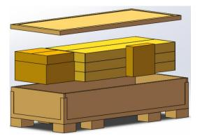
1 x 1\*4 box + 4 x 4\*1\*4 module packs + wrapped edges into honeycomb box, external dimensions: 2010\*870\*500mm
