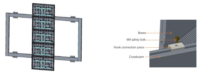
Note: The internal structure is based on the actual object.
