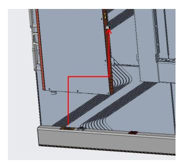
(3) Assemble the control box by following the control box slide
