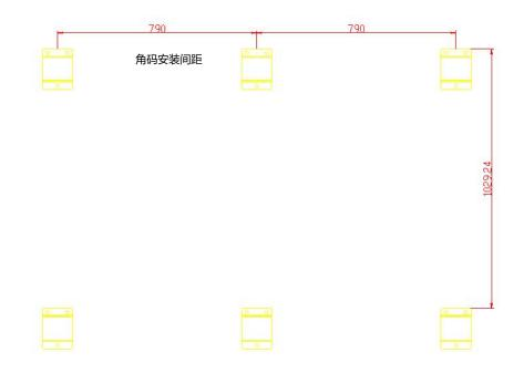
(2) After confirming the installation position of the fixed corner code of the back frame and the position of the screen, holes are punched in the wall to install the fixed corner code (only four corner codes can be installed on all sides when the wall has a better load-bearing capacity);
