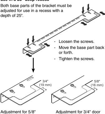
If the recess is deeper than 25", a spacer must be mounted between bracket and wall.
