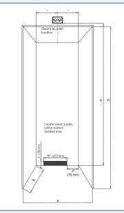
\*The given cabinet opening height dimension includes space for top air vent. If you choose to place the vent above the cabinet or in a soffit, you will need to adjust the height dimensions accordingly. Please refer to Ventilation Requirements.
