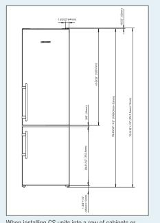
When installing CS units into a row of cabinets or wall units: Use these dimensions to achieve a custom look with the cabinetry while providing the necessary clearance for the top door hinge.
