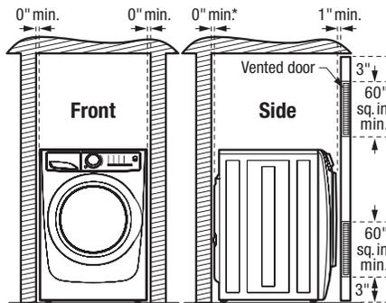
\*Installation with steam dryer requires additional 3/4" hose clearance.
