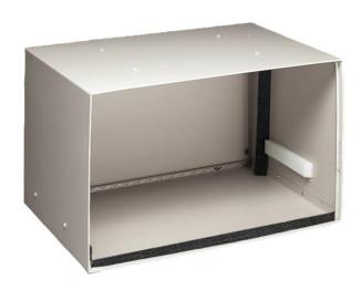
The Frigidaire EA108T is a Sleeve kit that is compatible with all Frigidaire Through-The -Wall Air Conditioners. It includes adjustable mounting brackets, lock clip, and inner sleeve seal. This kit is compatible with all FAH model Air Conditioners from 8,000 to 14,000 BTU.
